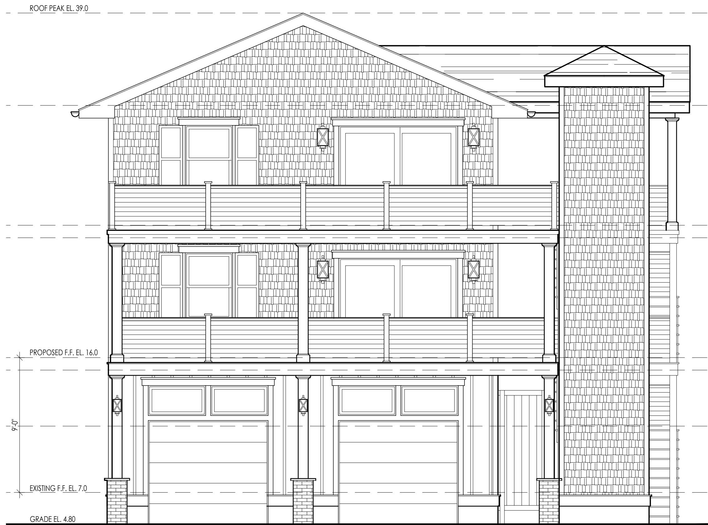
FRONT ELEVATION SCALE:1/4"=1'-0"
